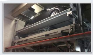
The Horizontal Puzzle Park is a fully automated system that utilises parking bed technology. The parking bed allows the system to move the vehicles parked on platforms in either a forward, reverse, left or right motion. This ability to move the platforms in any direction at any position allows the system to operate around corners, navigating the structure of the building and even shortening pathways for parking or retrieving vehicles.
